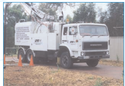
JETVAC equipment used to clean the RSF 4000
